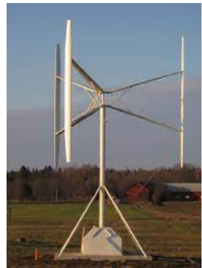
H-rotor design of a wind turbine (Reference: diva-portal.org )
