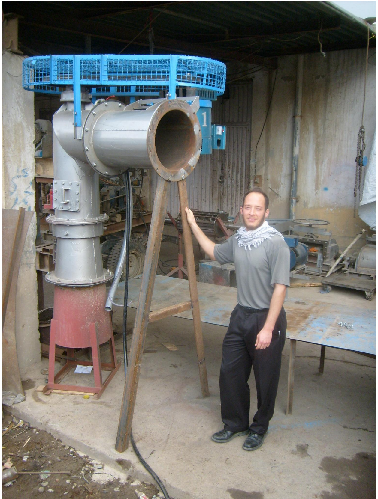
Figure 2 Photo of completed Kaplan turbine with short draft tube
