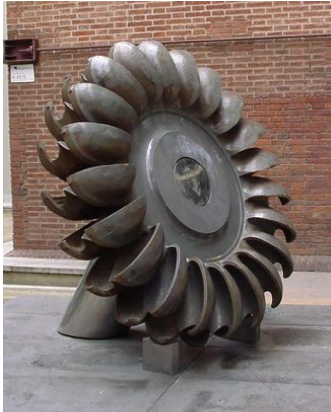
A Pelton Turbine (reference: energyeducation.ca)
