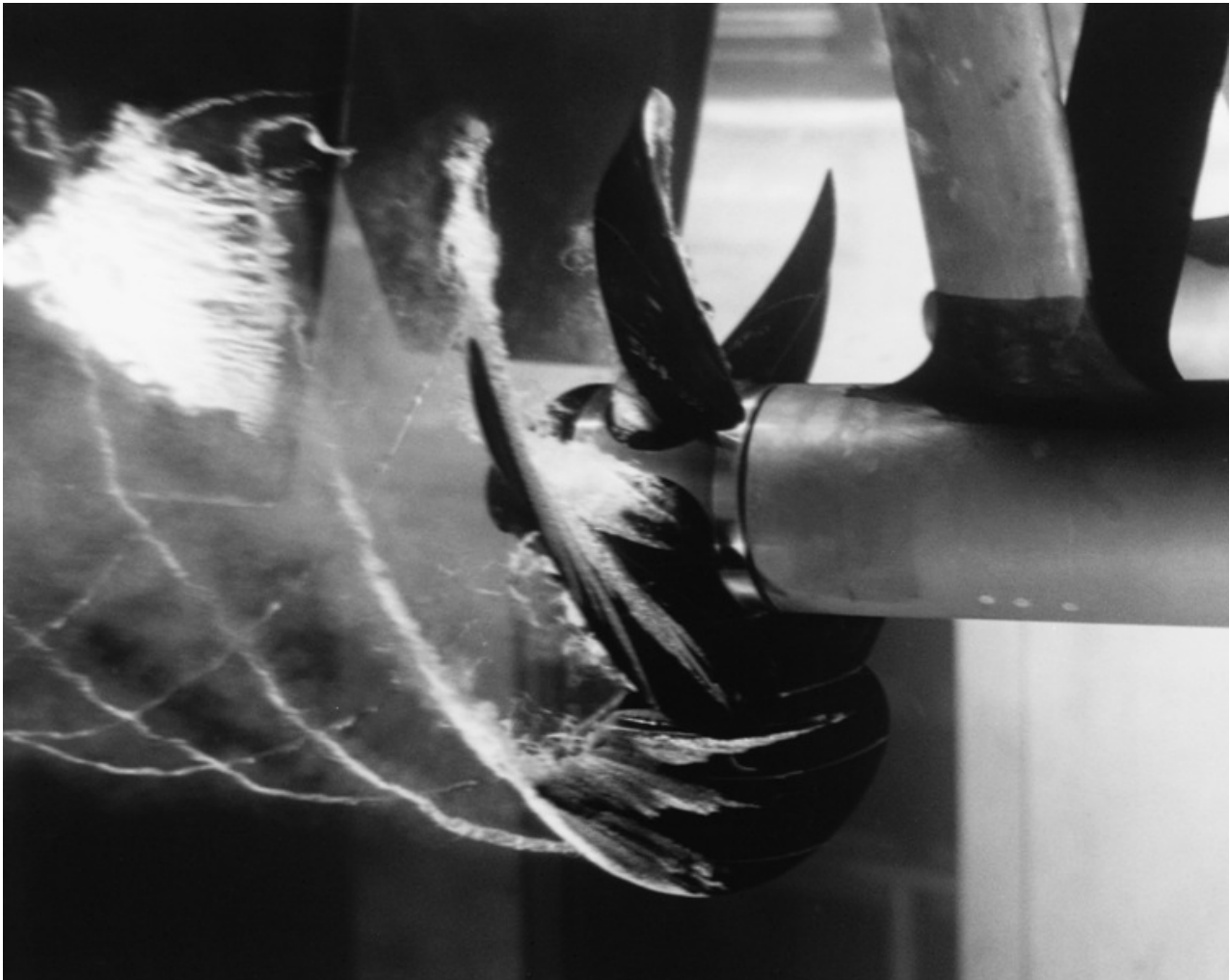
Cavitating propeller in water tunnel experiment (Reference: wikipedia.org )
