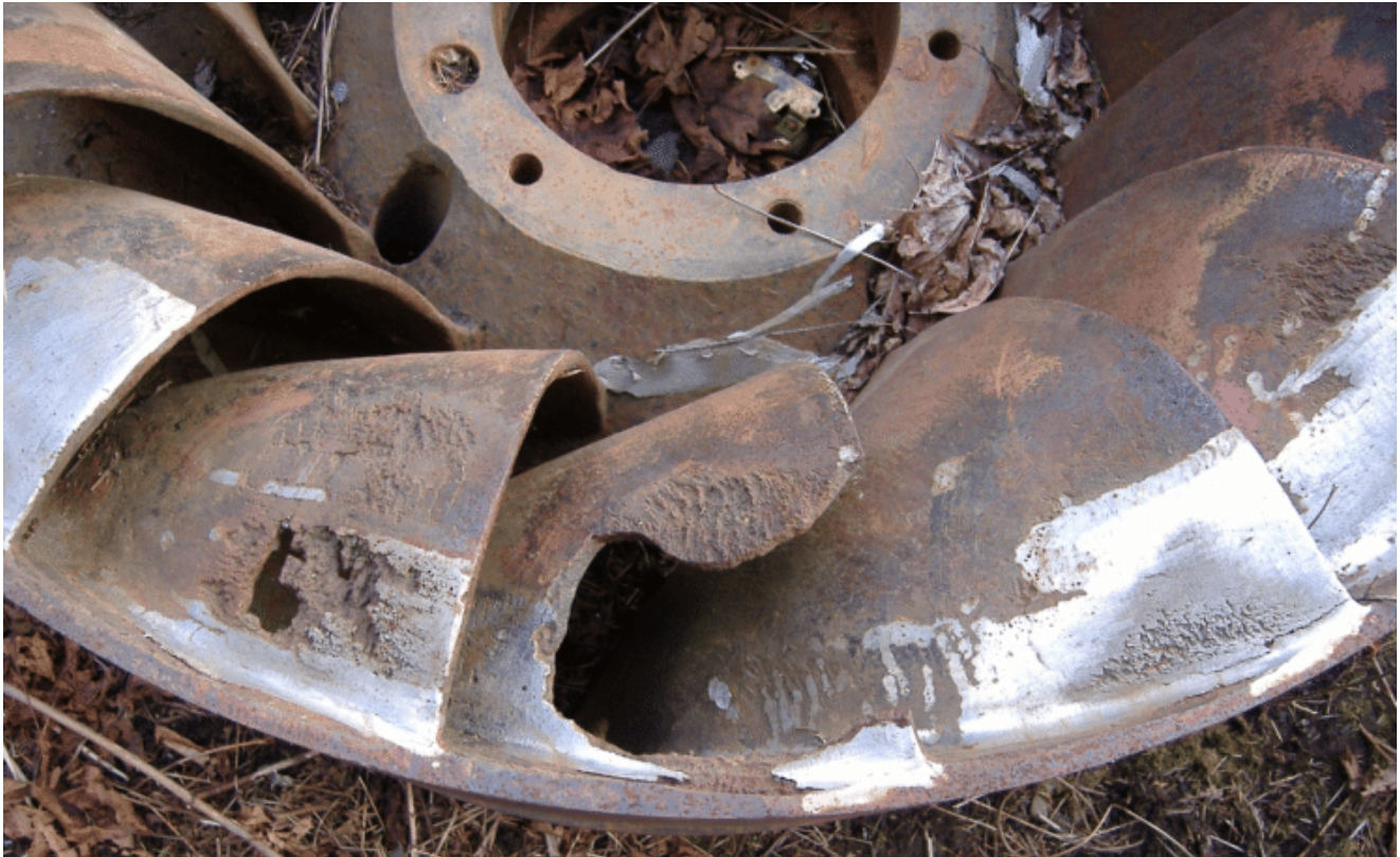
Cavitation damage to a turbine (Reference: researchgate.net )
