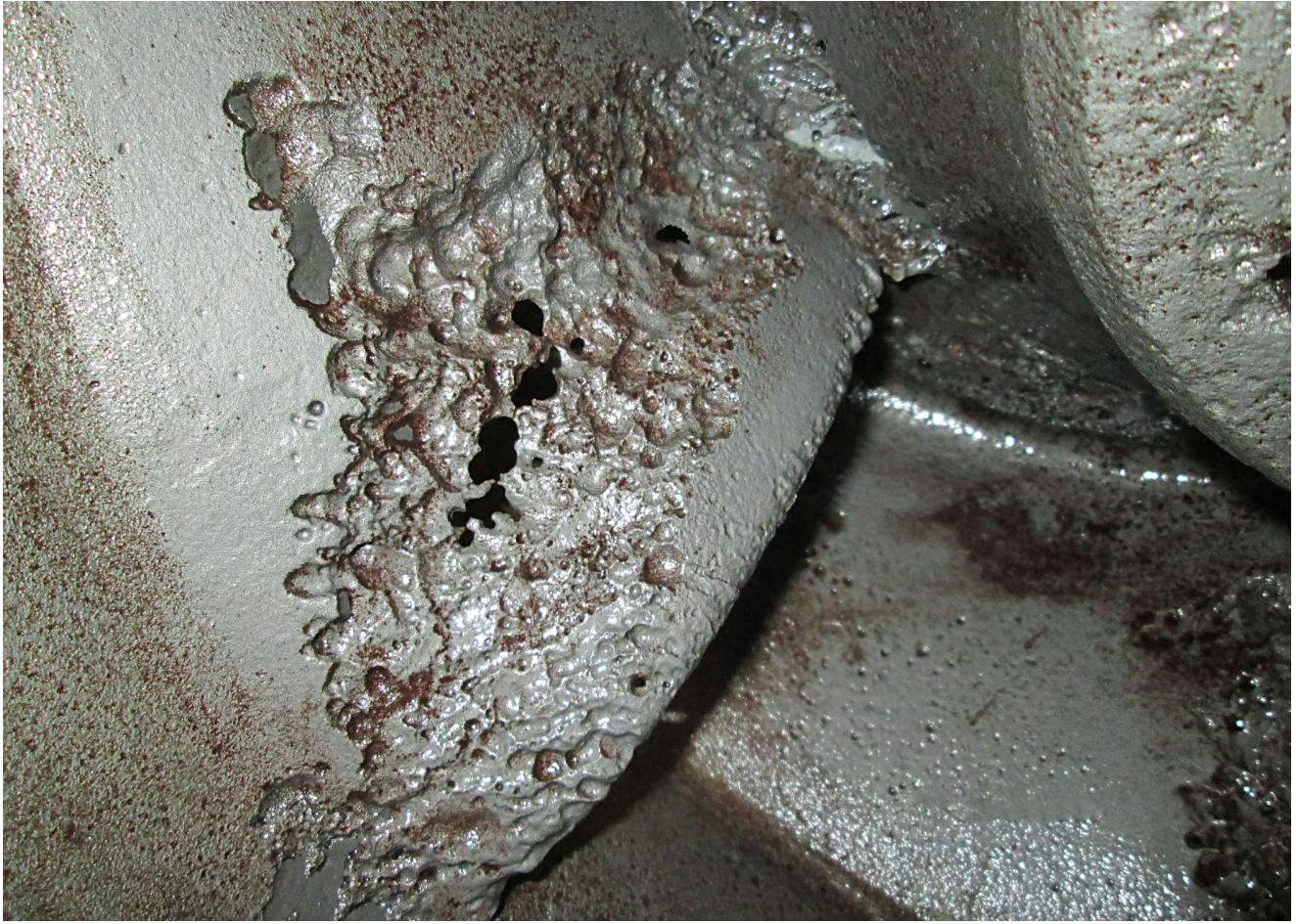
What cavitation brings to a pump (Reference: rodelta.com )
