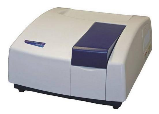
Double beam UV-visible spectrophotometer utilizes two monochromators, you can get two different wavelengths of monochromatic light. The two light beams alternately irradiate the same sample cell at regular intervals.
