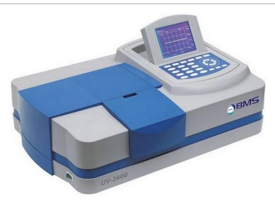
The light emitted by the same monochromator is split into two beams, one of which reaches the detector directly and the other passes through the sample and reaches the other detector. The advantage of this instrument is that it monitors errors in the light source, but does not eliminate the effects of the reference.
