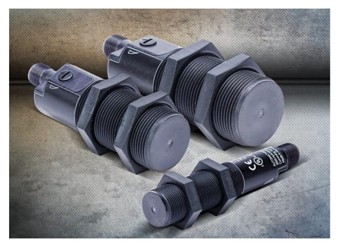
A proximity sensor is a sensor able to detect the presence of nearby objects without any physical contact. There are various types of proximity sensors out there in the market, but one can say this device often performs its object presence detection task by emitting an electromagnetic field or a beam of electromagnetic radiation ( infrared , for instance), and looking for changes in the field or return signal.
