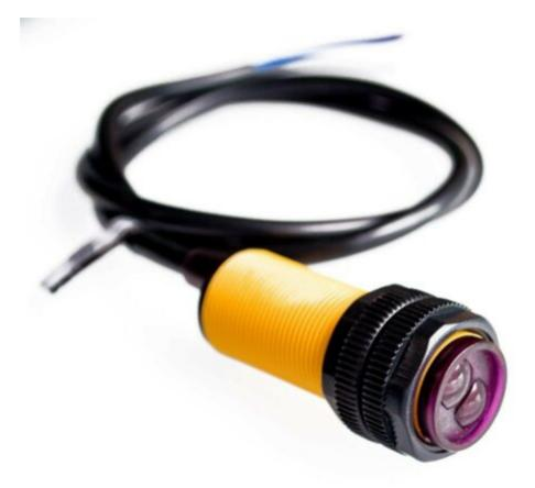
Infrared proximity sensors consist of an IR LED that emits, and a light detector for detection of reflection. It has an in-built signal processing circuit that determines an optical spot on the PSD.
