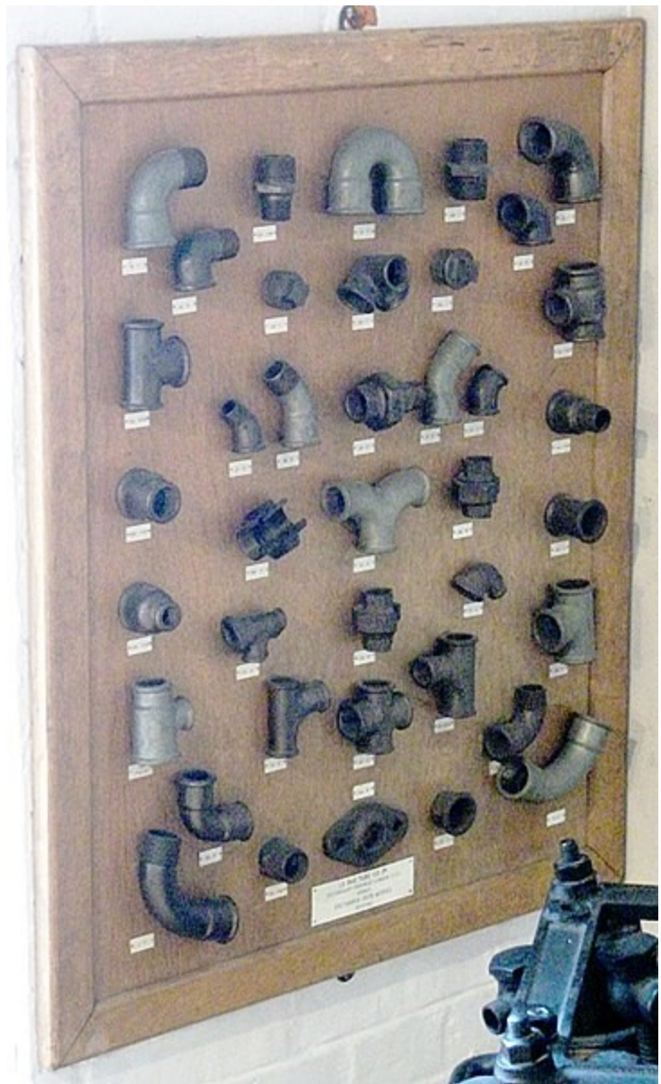
Example of threaded cast-iron fittings (Reference: wikipedia.org )
