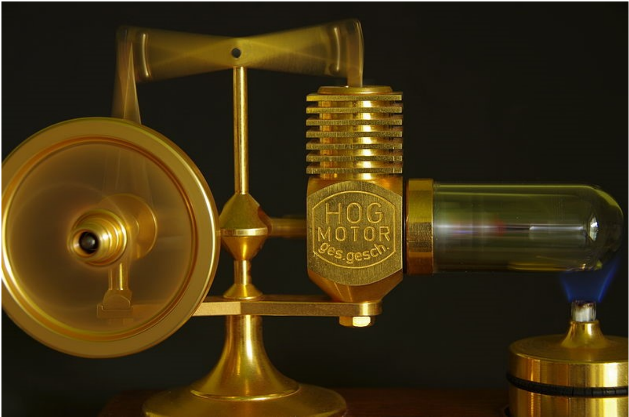
One of the first Stirling engine (Reference: wikipedia.org )
