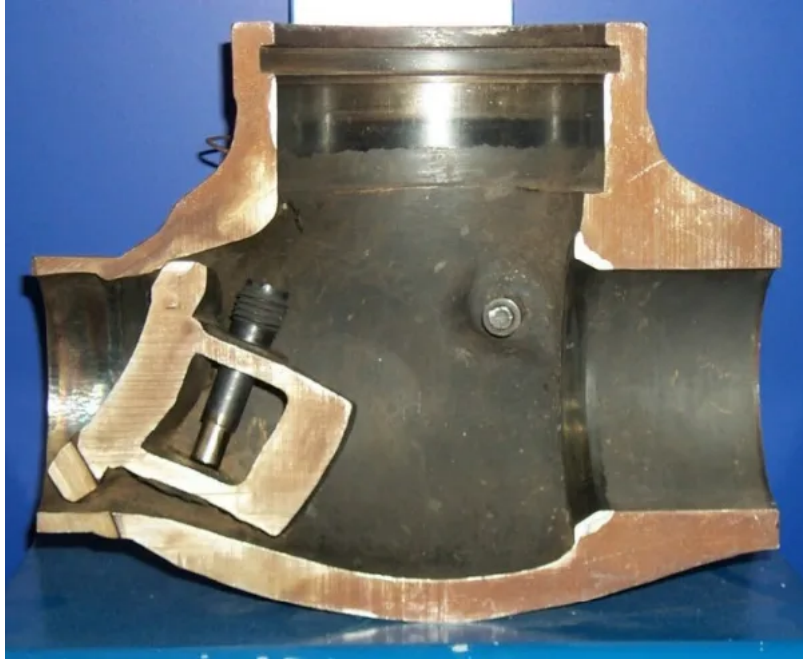
Wear and failure analysis of check valve (Reference: kalsi.com )
