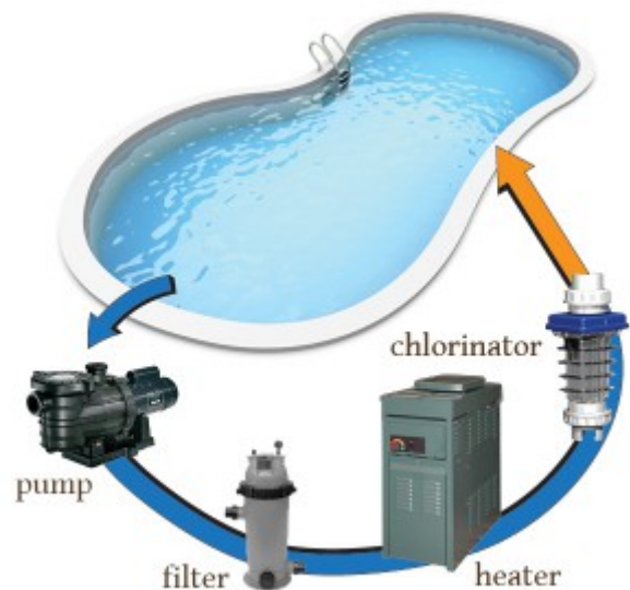
Working principle of a pool pump (Reference: inyopools.com )
