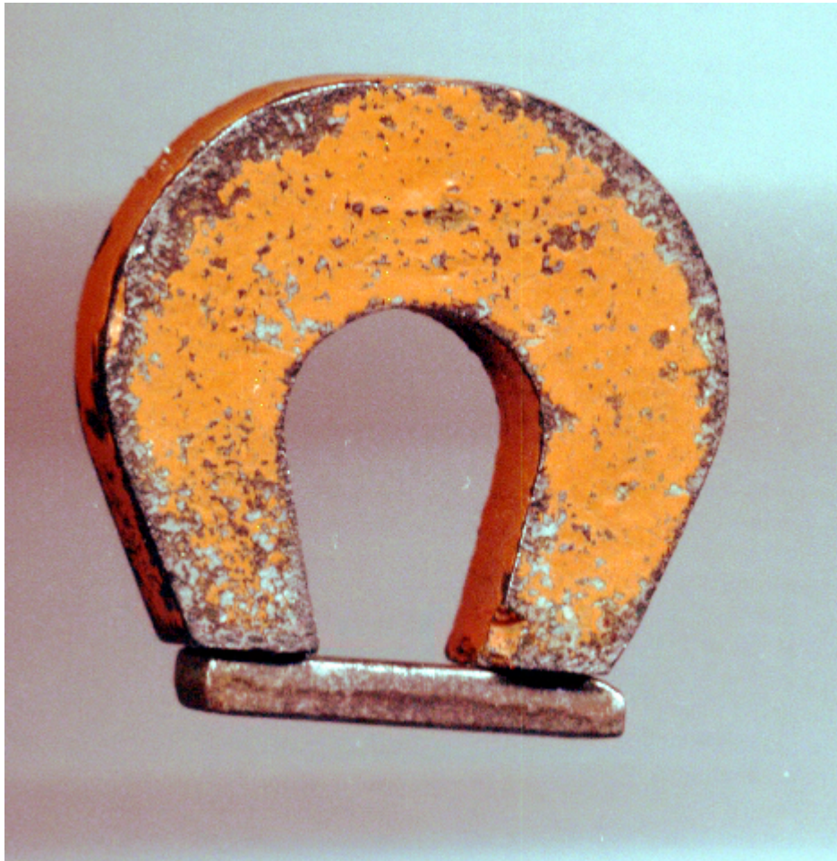
A “horseshoe magnet” constructed of the iron alloy alnico (Reference: wikipedia.org )
